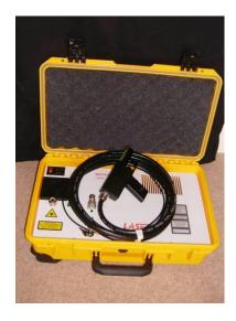
The Revelation Cordless single wavelength 577nm Yellow forensic laser from Laser Innovations Ltd is the latest compact laser in the Revelation family of products. With DNA cross contamination in mind this system is easy to clean with 10% bleach solution. The portable mains / battery operated laser system is designed for use in the Laboratory and / or the crime scene. This laser provides 3.5 Watts Blue at 577nm.
